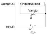
In applications where the inductive load is switched on and off frequently and/or rapidly, ensure that the continuous energy rating (J) of the varistor exceeds the peak load energy by 20 % or more.
