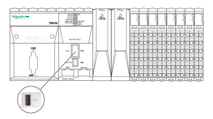
**NOTE:** The USB type A host port provides 500 mA continuous current (USB-standard) and 700 mA for short duration current spikes.
