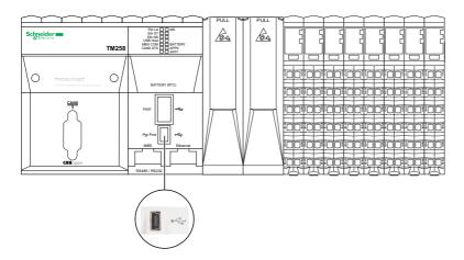
The USB Mini-B Port is the programming port you can use to connect a PC with a USB host port using EcoStruxure Machine Expert software. Using a typical USB cable, this connection is suitable for quick updates of the program or short duration connections to perform maintenance and inspect data values. It is not suitable for long-term connections such as commissioning or monitoring without the use of specially adapted cables to help minimize electromagnetic interference.
