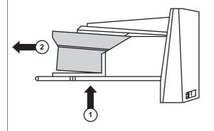
4 Insert the new battery into the battery holder in accordance with the polarity markings on the battery:
