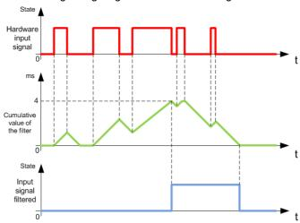
**NOTE:** The value selected for the filter's time parameter specifies the cumulative time in ms that must elapse before the input is recognized as logical 1, as well as specifying how long the filtered input signal remains at logical 1.
